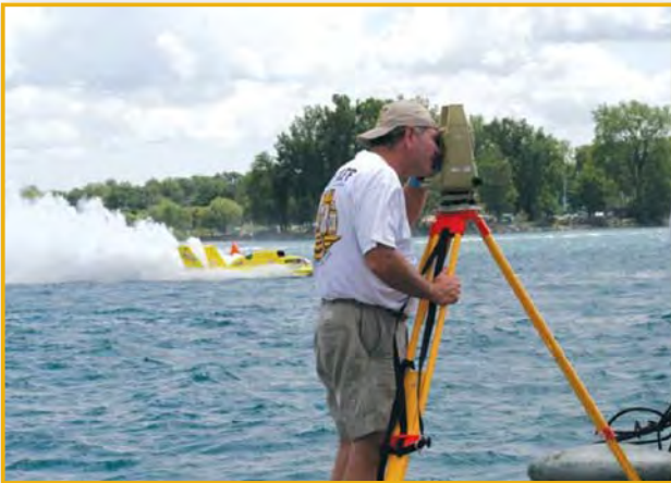
MSPS Southeast Chapter President Jim Hollandsworth, PS, uses a Leica TC 600 to verify the course from station five near the final turn while one of the unlimited hydroplanes performs a qualifying lap. Photo by Reed Zapf.
